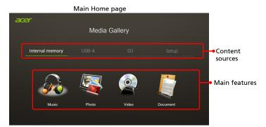
This mode allows you to browse media files stored in different devices, such as RAM (internal memory), USB flash drive, USB hard drive and SD card (for selected models) when connected to the projector. No matter where you are, you can always press MEDIA HOME to go back to MEDIA HOME page.
